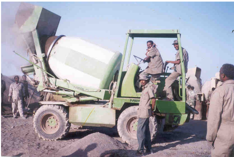
Figure 6 Movable concrete mixer utilized at Assab hospital.
