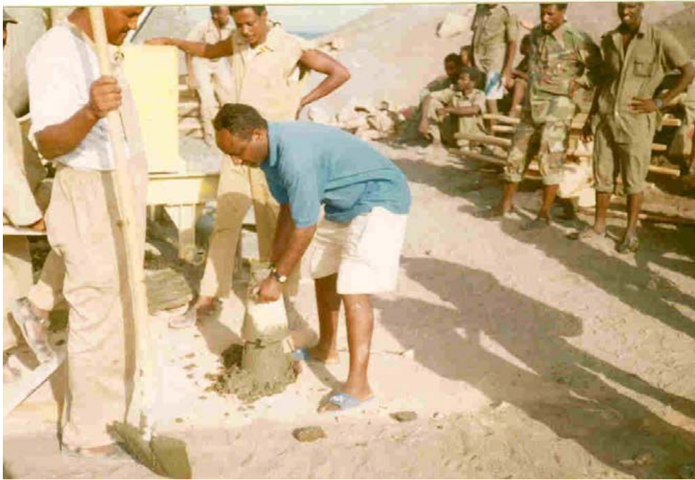
Figure 7 Slump test.
